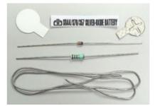
A \*625-kit comes with a BAT83 Schottky diode (DO-34); if another diode is required (see page 4) include this in your order. The kit also contains a  $100\Omega$  (Ohms) resistor for draining the alkaline cell, a pre-cut isolating self-adhesive sticker and a (metal) pre-cut solderable conductive self-adhesive sticker, 2 preprinted isolators (plastic-coated paper) with cell type and battery placement instructions on it and a piece of solder. Ordering information can be found on page 11.
