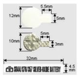
A conductive and solderable self-adhesive tinned copper shielding foil, made by 3M, type 1345, cut in the shape as shown on the left. This foil is intended for shielding of components from R.F. and E.M.C. signals. It is expensive material and often hard to get. Look for
